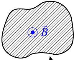
**Faraday's Law:** The induced emf due to a changing magnetic field is equal in magnitude to the rate of change of the magnetic flux through a surface bounded by the circuit. The direction of the induced current is given by Lenz's Law.
