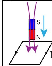
**Lenz's Law:** The current induced by a changing magnetic flux creates a magnetic field opposing the change in flux.
